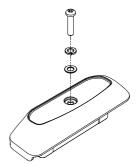
Tighten the screw with the allen key provided. **Do not over tighten.**
