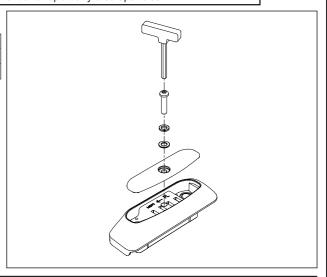
When the crossbars have been removed from the mounting pads, place the cover into the mounting pad recess.
