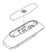
Assemble the spring washer and flat washer onto the leg attachment screw used to attach the leg to the mounting pad. Insert the screw assembly thought the cover plate hole and screw into the mounting pad.
