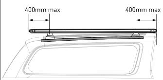
NOTE: For 4XXXX series Pioneers, additional Ø8.5mm holes may need to be drilled into the side extrusion to allow pioneer underbars to align with the legs
