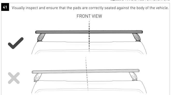
Tighten bolts **incrementally** and **evenly** on each side of the vehicle to avoid pulling the rack to one side.
