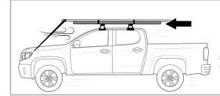
Long flexible loads must be securely attached to a rigid **support** and be tied down to the bonnet.
