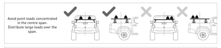
The handling characteristics of the vehicle changes when a load is transported on the vehicle exterior.
