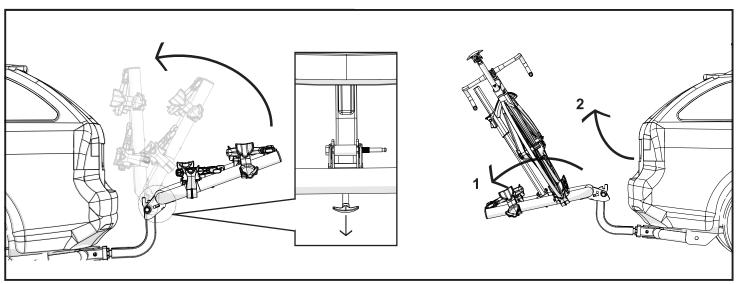
Gently release handle to raise and lower rack into stow, use, and tilt positions. Rack can be folded into stow position when now in use and tilted down for rear vehicle access. Load arms should be stowed flat when rack is not in use. Handle should be fully seated before each use.
