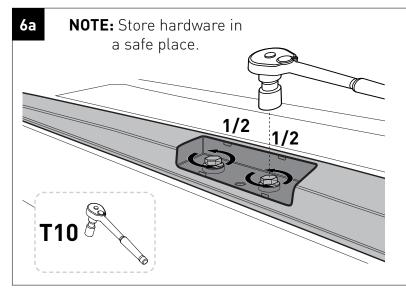
Break both bolts loose, incrementally turning each a half turn at a time, until they are both loose enough to remove by hand.
