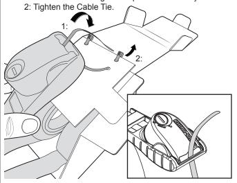
Using Cutters, remove the excess Cable Tie.
