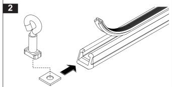
Position the Ladder peg, then tighten to secure. It is very important that the Channel nut is fully located across the cross bar. Trim the rubber buffer strip to fill the gap either side of the Ladder peg.
