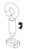
Remove rubber buffer strip. Slide the Eye bolt base with the recess facing up into the top of the cross bar. With the Ladder peg and Channel nut attached slide into the top of the cross bar.
