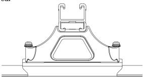
Tighten all leg bracket attachment bolts. Adjust the crossbar for equal overhang each side of the vehicle as per the diagram. Tighten all crossbar attachment bolts.
