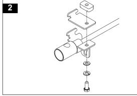
Check that the lock housing is facing the rear of the vehicle, turn the channel nut so that the channel nut is fully located across the crossbar.
