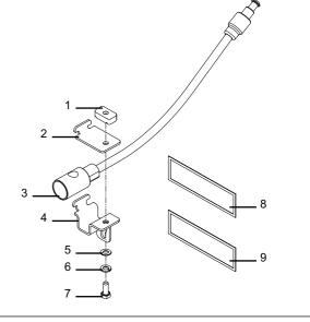
Unlock the cable lock, align the flats on the cable lock with the flats on the lower bracket and insert the cable lock into the lower bracket. Ensure the cable lock housing is fully located into the bracket.
