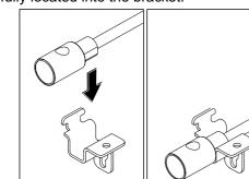
Insert the T-shaped lugs on the brackets into the underside of the crossbar. Turn the cable lock and bracket assembly so that the lugs engage the crossbar and the channel nut goes up into the crossbar recess.
