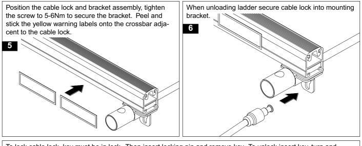
To lock cable lock, key must be in lock. Then insert locking pin and remove key. To unlock insert key, turn and remove locking pin.
