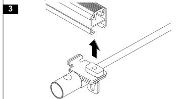
Assemble the nut, screw, washer and upper bracket. Place the upper and lower brackets together, screw on the channel nut, one turn, and align the channel nut.
