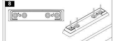
Place the fixed mount bracket into the pad location spigots. Assemble the spring washer and flat washer onto the M6 screws. Insert the screws through the pad spigot holes and tighten to secure the fixed mount base plate.
