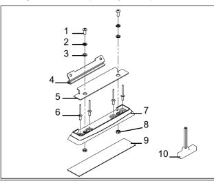
Place the fixed mount pads onto the roof with the cut out section facing outwards. Position the pads so that the pads are parallel to each other, inline and square across the roof.
