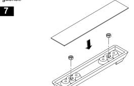
Clean the gasket face to remove dirt. Place the pad onto the roof and insert the four rivets through the pad and into the roof. Check that the pad cut out is facing outwards and the rivets are seated in the pad. Using either a pneumatic or concertina type rivet gun, rivet the pads into place starting from the centre and working out. Check that all rivets are seated firmly into the pad.
