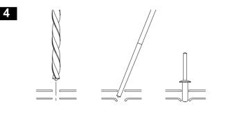
Make sure to remove all swarf with a vacuum cleaner. This prevents rust from occurring as a result of residue swarf.
