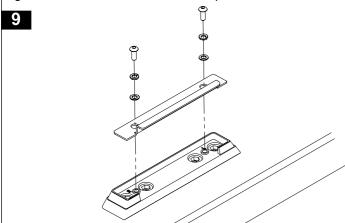
Assemble the strap provided onto the leg assembly. Discard the existing strap. Install the rubber boot then locate the leg against the fixed mount leg bracket. Rotate the strap and cover so that the strap is fully located under the bracket. For tightening and checking of the leg and crossbar please refer to the Rhino gutter mount leg fitting instruction.
