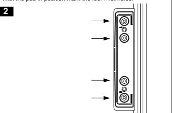
Remove the pads, centre punch the centres. Drill all holes using a 5.0mm drill bit. When drilling, a drill stop should be used to ensure that only the outer roof panel is drilled.
