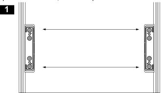
With the pad in position mark the four rivet holes.
