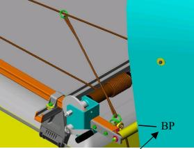
The (BP) balance point ' must be at the pivot roller to maximum of 50mm below the pivot roller.
