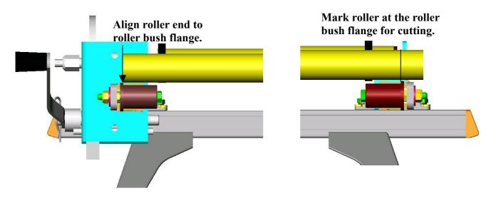
Remove burrs and clean the cut end of the roller. Remove the pivot roller bracket from the driver side longitudinal bar, insert the pivot roller into the winch side bush, insert the driver side bracket bush into the roller. Insert the pivot roller bracket into the longitudinal bar, adjust the pivot roller to be parallel to the power roller.
