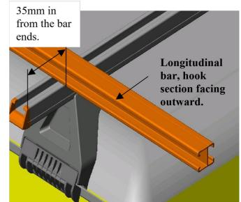
Minimum bar overhang to fit the winch.
