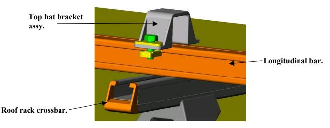
Check that the passenger side bar is still parallel. Tighten only the rear crossbar top hat bracket. Note: when tightening bolts with channel nuts, ensure that the channel nut is fully located across the crossbar recess when fully tightened. (Refer Diagram).
