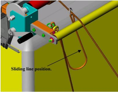
The position of the sliding lines should be between the pivot roller and power roller, as per the diagram.
