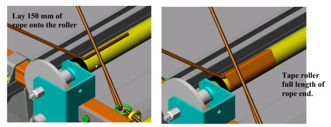
Turn the winch handle clockwise, winding the rope coils inward and over the taped rope end covering the full length of the tape, ensure there is tension on the ropes and the rope coils are tight and together. Tape over and around the rope coils for the full length of the coils ensuring overlapping of the tape, put three layers of tape over the coils, as per the diagrams.
