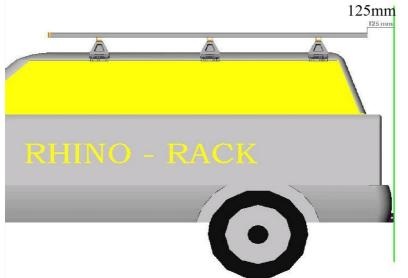
Position the passenger and driver longitudinal side bars 35 mm in from the ends of the crossbar and 125 mm from the extreme end of the vehicle to the end of the longitudinal bar, including the spare wheel carrier if fitted. Refer Diagrams.
