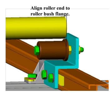
Remove burrs and clean the cut end of the roller. Assemble two sleeves and four rubber rings onto the roller as shown. Remove the un positioned Z bracket, insert the front roller into the fixed Z bracket bush, and insert the other Z bracket bush into the roller. Insert the Z bracket into the longitudinal bar, adjust the front roller parallel to the power roller. Tighten the attachment bolts as previously described and check that the channel nuts are fully located across the bar.
