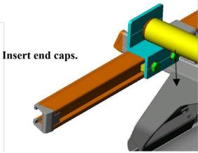
Position front crossbar assembly against the front roller Z brackets check that the crossbar is parallel to the rear crossbar.
