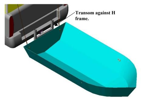
Clip both tie down line snap hooks onto the transom eye nuts. The bottom of the boat may be required to be lifted of the ground to attach the hooks, do one side at a time.
