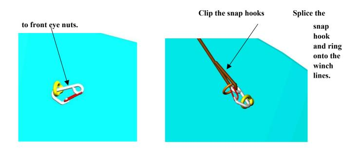
With all snap hooks connected to the eye nuts the boat should be balanced on the keel. If the winch lines are of unequal length, the boat, when in the vertical position will be leaning and will skew on the rollers.
