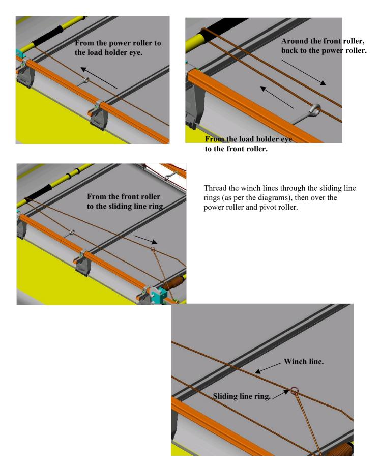
Take both ends of the winch lines and pull to tension the lines. With tension on the lines turn the winch clockwise 5 turns, the lines will coil inwards.
