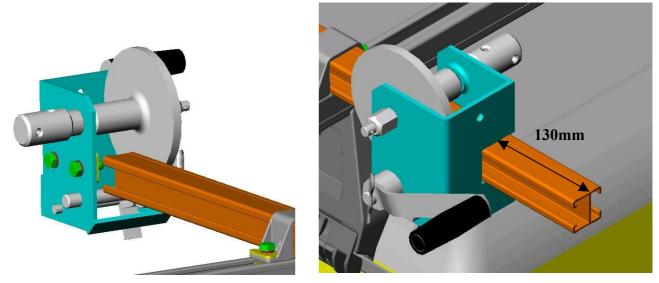
Check the channel nut is fully across the bar.
