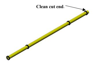
Remove burrs and clean the cut end of the power roller, slide the rubber rings onto the roller in any position. Place the rings in hot water, this will aid the rings to slide onto the roller.
