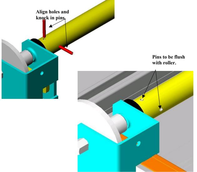
When fitment of the power roller is complete, rotate the winch and check that the winch and roller rotates freely.
