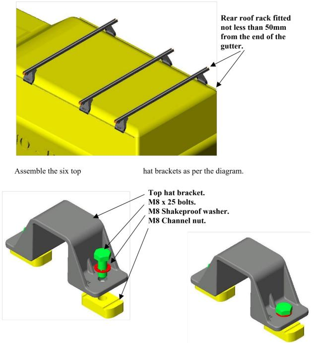
Place the longitudinal bars onto the crossbars with the hooked section of the bars facing outward. (Refer Diagram).
