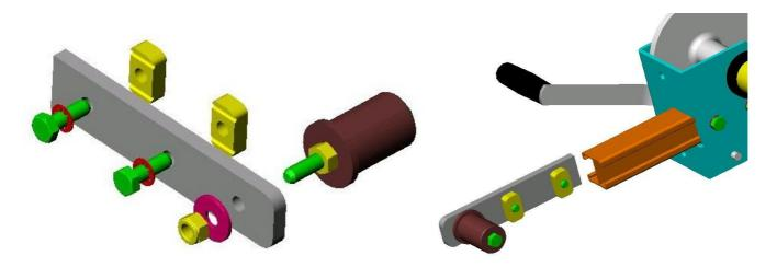
Slide the winch side pivot roller bracket into the longitudinal bar so that the end of the bracket is against the winch with the roller bush facing inwards. Tighten the attachment bolts; **check that the channel nuts are located fully across the bar.**
