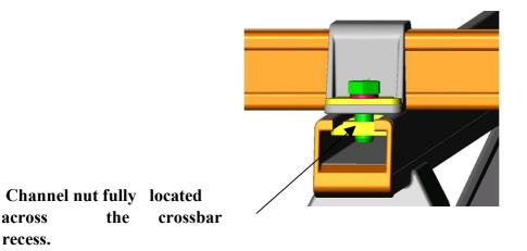
Position the driver side longitudinal bar, parallel to the passenger side bar, the end of the bar should be the same distance from the crossbar as the passenger side bar. (Refer Diagram). Tighten the rear crossbar top hat bracket only. (Refer Diagram).
