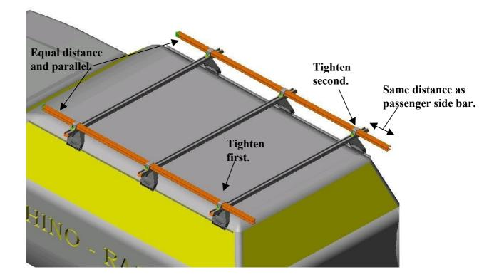
The two front top hat brackets can be tightened to hold the longitudinal bars in place while the rollers are being positioned and cut.
