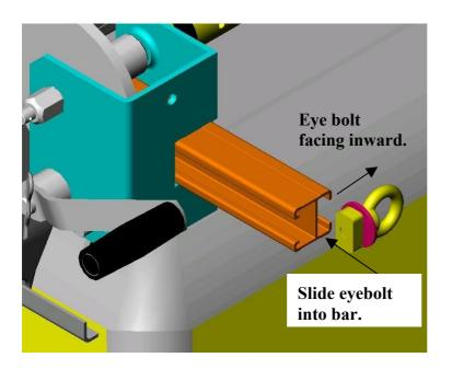
Position the eyebolt washer level with the end of the longitudinal bars. Tighten the eyebolt and check that the channel nut is fully located across the bar. When tightened, the eyebolt must be vertical.
