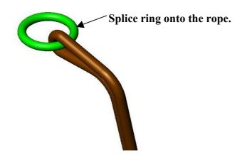
Mark a length from the ring to the free end of the rope equal to the distance from the transom to the balance point, a piece of masking tape around the rope will do to mark the distance.
