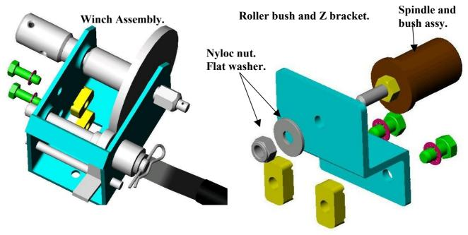
Slide the winch onto the passenger side longitudinal bar with the winch handle facing outwards, as per the diagram. Position the winch 130mm from the end of the bar. Tighten the attachment bolts, **check that the channel nuts are fully located across the bar**.
