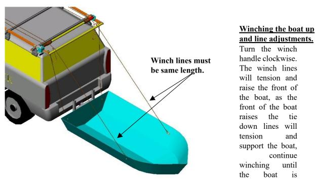
vertical and the gunnels are against the pivot roller. Check that the balance point marked on the boat is inline with the pivot roller to a maximum of 50mm below the roller, if the position is incorrect lower the boat and adjust the tie down lines by un-splicing, move the snap hook and splice. Recheck the balance point to pivot roller before winching further.
