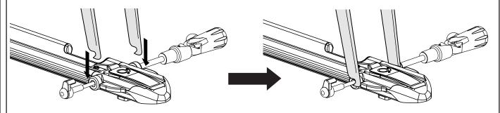
Twist handle clockwise to tighten the quick release skewer. Close the handle by flipping it 90 degrees to the closed position. If it is too loose, open the handle and turn it like a screwdriver (clockwise to tighten, counter clockwise to loosen), and close the handle again. Re-adjust until a firm and positive snap is felt when closed.
