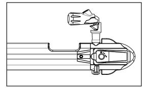
Open the handle of the quick release so the black handle is straight and the fixed end points down. Load the fork onto the quick release so both fork ends are resting straight on the quick release.
