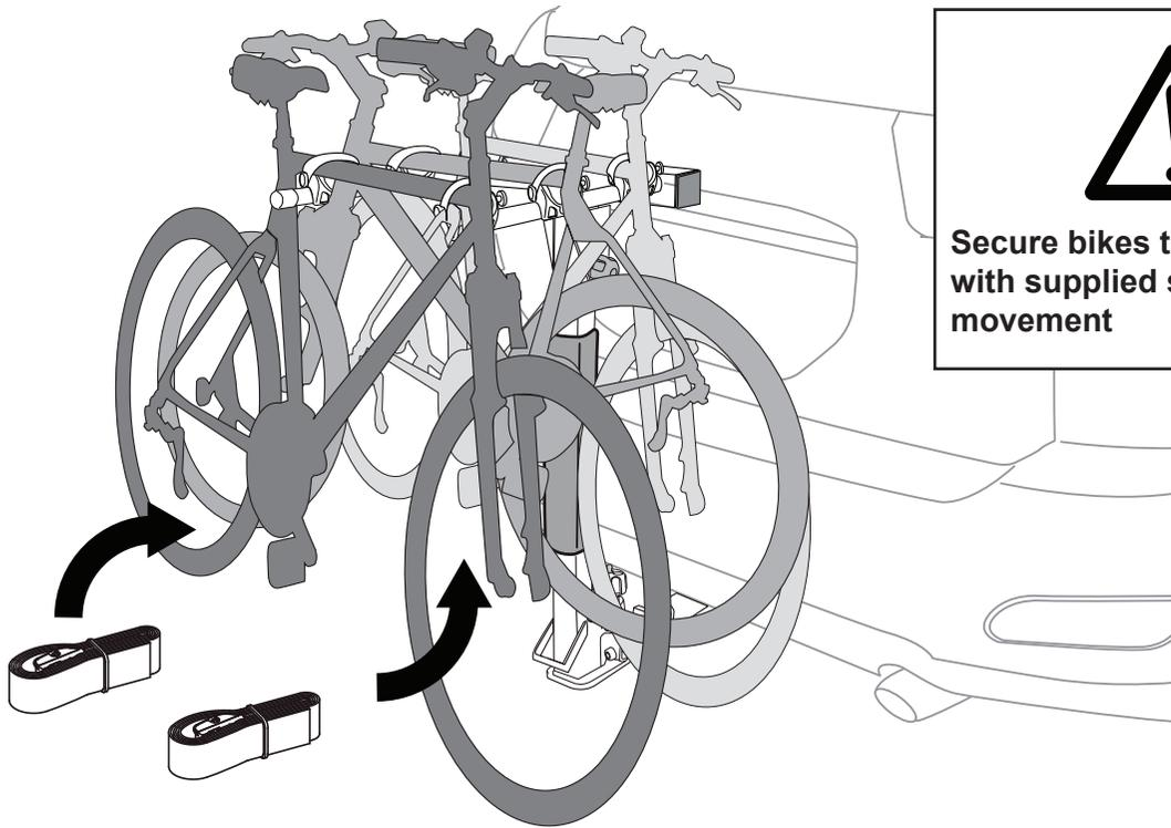
**Secure bikes to bike carrier with supplied straps to avoid movement**
