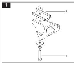
Remove the M10 x 25mm bolt. Re-fit with the Leg Offset Spacer and longer M10 x 35mm bolt along with the existing washers and channel nut. Install the cross bar and leg as normal.
