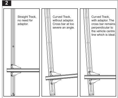
The Leg Offset Spacer allows cross bars to be mounted perpendicular to the vehicle centre line on tracks that curve towards the front or rear of the vehicle. The adaptor allows a maximum rotation of 5° while still maintaining sufficient load bearing area.
