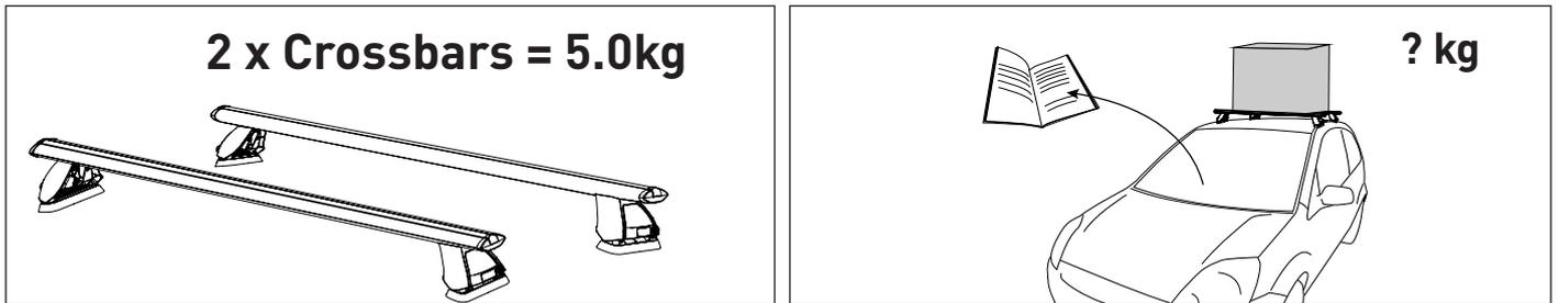
When these roof racks are to be used on a vehicle that is driven off sealed roads, the manufacturer maximum roof load rating (to be found in the vehicles User Manual) should be **halved**. Do not forget to subtract 7.5kg from your maximum carrying capacity due to the weight of the crossbars and legs.
