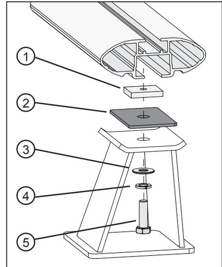
**1** Fix the M6 x 20mm Hex Bolt, both Washers, 2mm HDPE Spacer and M6 Plate Nut onto the EGR post as shown.
