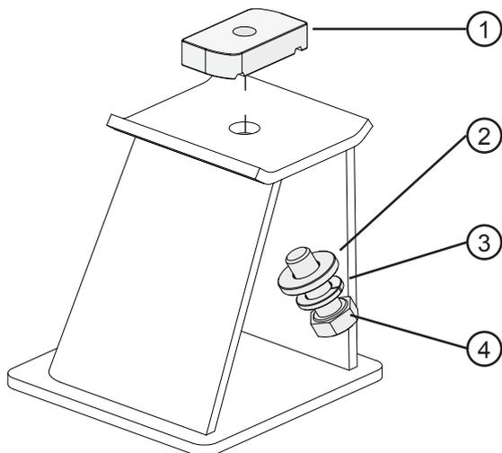
**2** Slide Rhino Heavy Duty Bar onto channel nut as shown and tighten with the 13mm Spanner.
