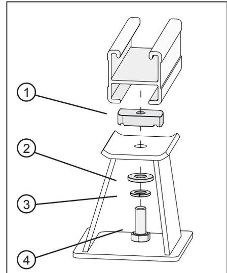
**1** Fix the M8 x 20mm Hex Bolt, both Washers and M8 Channel Nut onto the EGR post as shown. Make sure the channels on the M8 Channel Nut are facing downwards.
