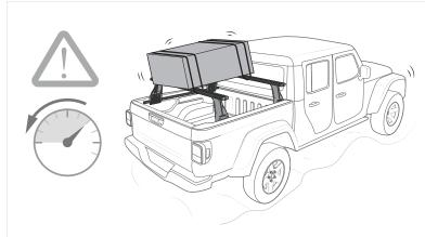
The handling characteristics of the vehicle changes when a load is transported on the vehicle exterior.
