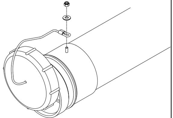
With the hex bolt pointing up place the warning label 90 degrees to the hex bolt.
