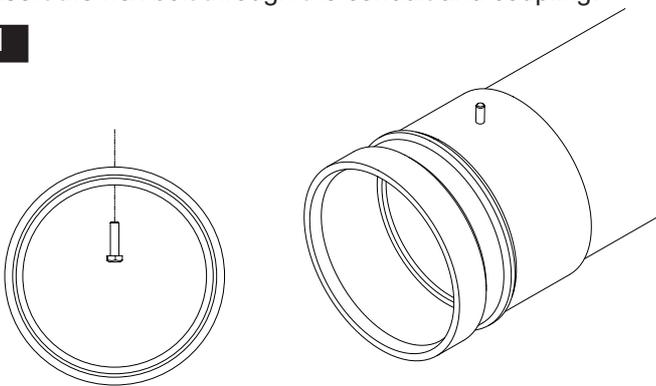
Place the wire trace over the hex bolt, assemble the flat washer and nyloc nut. Tighten the nyloc nut.
