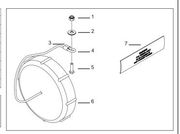
Insert the hex bolt through the conduit and coupling.
