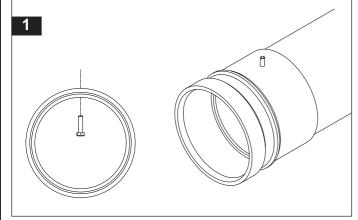
Place the wire trace over the hex bolt, assemble the flat washer and nyloc nut. Tighten the nyloc nut.
