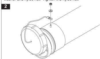
With the hex bolt pointing up place the warning label 90 degrees to the hex bolt.
