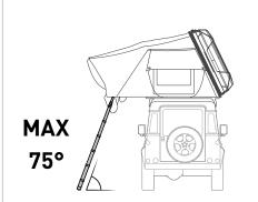
Inclination angle should not exceed 75 degrees.
