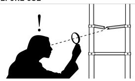
Inspect operation of ladder locks, rungs and telescopic parts before use each time. Do not use if damaged.
