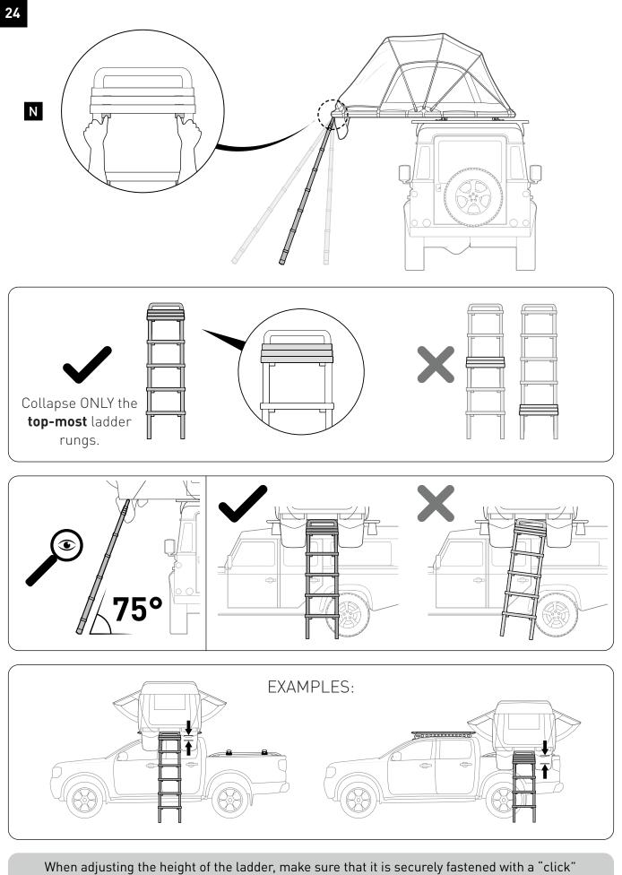
When adjusting the height of the ladder, make sure that it is securely fastened with a "click" CHECK LADDER RUNGS ARE LOCKED IN PLACE BEFORE ATTEMPTING TO CLIMB LADDER
