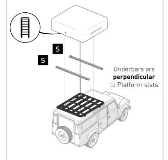
The underbars are **pre-installed** for Rear Opening tents on Platforms
