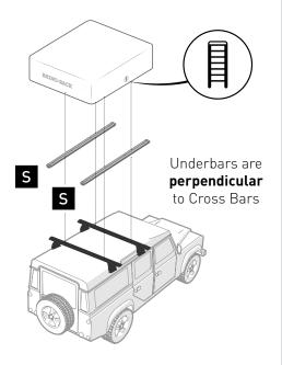
The underbars are **pre-installed** for Side Opening tents on Cross Bars.
