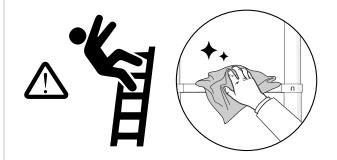
Remove any slippery contaminants from the ladder rungs such as mud, oil, grass or snow to ensure a secure grip.
