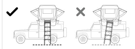
Ladder should be positioned on an even, level and unmovable surface.
