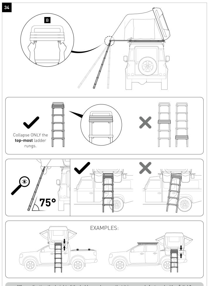
When adjusting the height of the ladder, make sure that it is securely fastened with a "click" CHECK LADDER RUNGS ARE LOCKED IN PLACE BEFORE ATTEMPTING TO CLIMB LADDER
