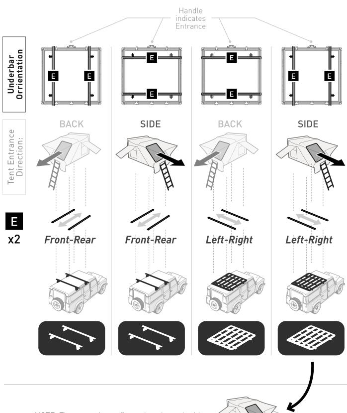
NOTE: The example configuration shown in this instruction is **Side opening** on a **Platform**
