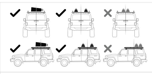
Distribute loads evenly and longitudinally as low as possible over the span.
