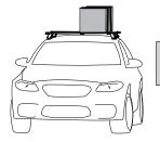
60kg load rating (Urban road) = 30kg load rating (Off road - 60kg / 2)
