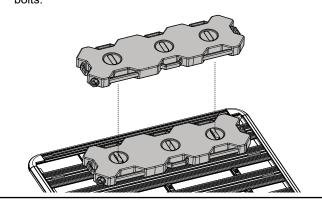
Ensure that the upper handle tightened and is positioned perpendiuclar to the lower handle.
