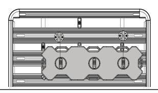
Place the Rotopax onto the pack mounts. Tighten all four
