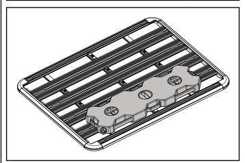
Assemble the bracket kit as shown. Do not tighten hardware at this stage.
