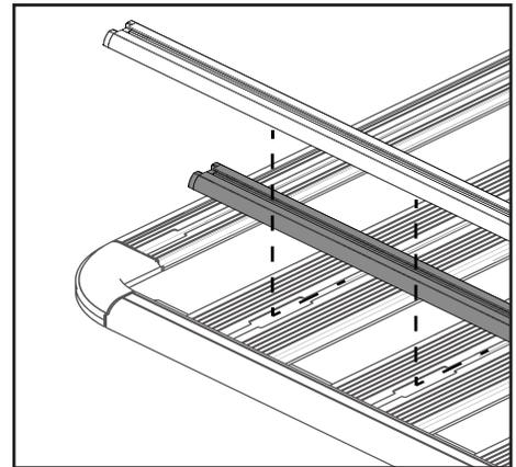
**3** Make sure the channel nut is located across the plank as shown.
