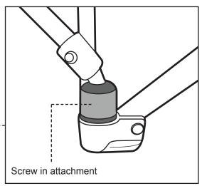
Unscrew the foot rest attachment and remove from both front legs of the chair.
