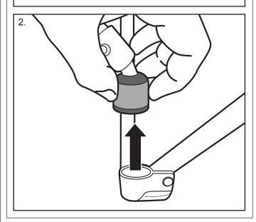
B Detach the foot rest clips and remove the foot rest.
