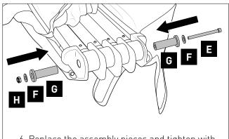
6. Replace the assembly pieces and tighten with **T1** 6mm Allen Key and **T3** 13mm Socket Wrench.
