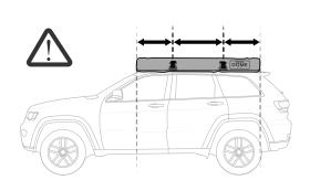
NOTE: Ensure Awning has close to equal overhang over Front and Rear crossbars.
