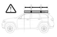
**NOTE:** Ensure Awning has close to equal overhang over Front and Rear crossbars.
