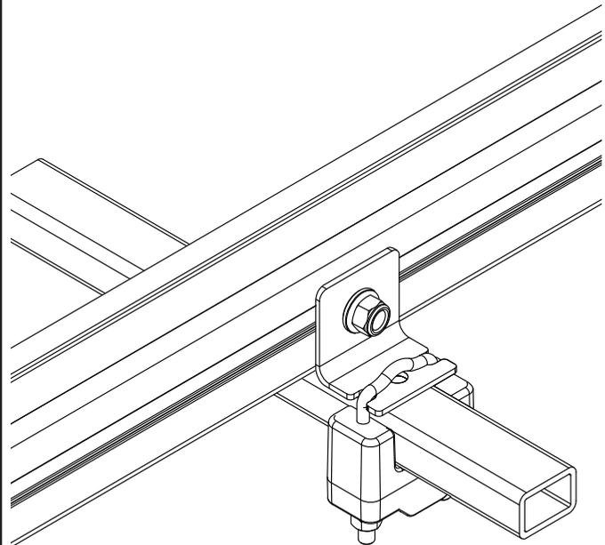
**Tighten to 4-5Nm. Check fitting regularly.**
