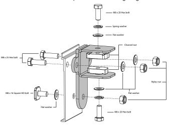
4 Slide the assembled Fiamma awning bracket unit into the 'C' Channel of the HD bar. Tighten all bolts.
