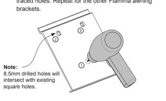
Assemble the hardware onto each of the Fiamma awning brackets with the adapter as shown. Finger tighten.
