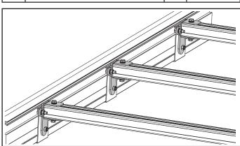
Place the awning bracket on a Fiamma adapter that is secured to the awning such that the bottom hole of the awning bracket is in line with the middle of the bottom channel spacing. Mark the holes using a pencil onto the adapter.
