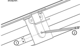
Using a drill with a 8.5mm drill bit, drill through all three traced holes. Repeat for the other Fiamma awning
