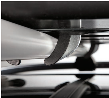
Jaws tighten around crossbar.
