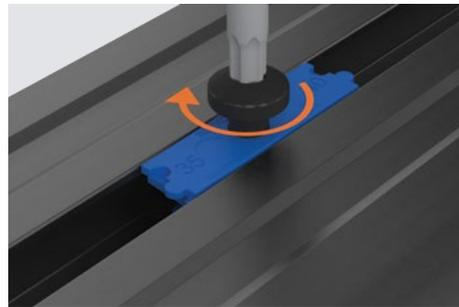
Tighten the bolt to engage.
