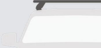
An overhang system creates additional storage space where the ends of the cross rails sit further out than the mounts.
