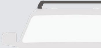
A flush system is both sleek and stylish in design where the cross rails do not overhang the mounts.
