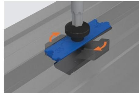
High tensile M6 nut rotates within the housing cage to lock in under the channel lip.
