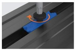
Tighten the bolt to engage.
