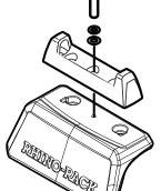
Install RLT600 Base kit to the castings utilising M6 hardware supplied in leg kit.
