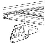
Attach leg assemblies to the Pioneer underside bars. Tighten leg hardware to a firm <u>sliding</u> fit.
