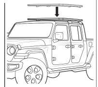
Place Pioneer assembly onto RJTB1 castings. Slide legs into position and attach to castings. Centre Pioneer between legs and tighten all hardware to final torque.
