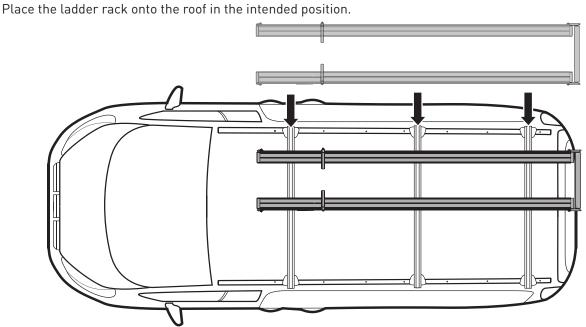
Be sure the rear of the CSL ladder rack, clears the rear of the vehicle but does not contact an open rear door.
